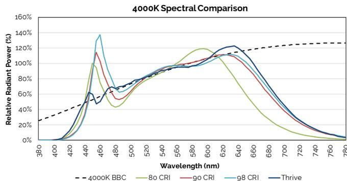
**SMD 2835 0.2W, 3V Thrive Pulsed Measurement Data, T<sub>sp</sub>=25°C**
