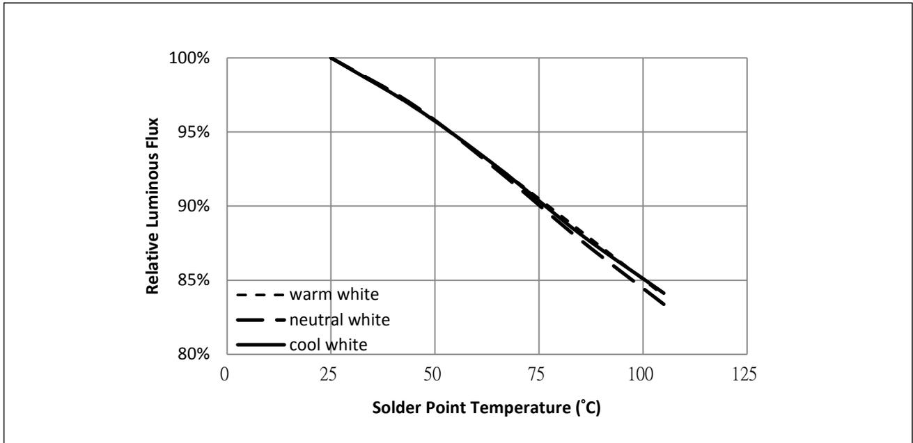
**Figure 5: Typical ccx Shift vs. Solder Point Temperature**
