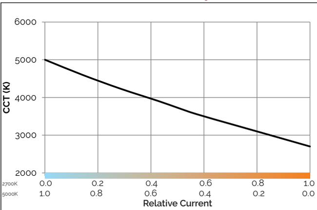
**Figure 11: CCT vs. Relative Current,  $T_c = 85^\circ\text{C}$**
