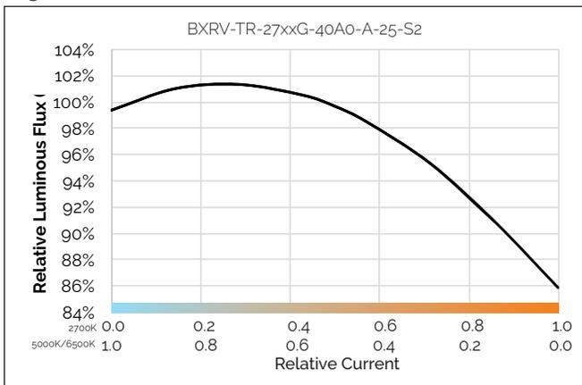
Figure 17: Relative Flux vs. Relative Current
