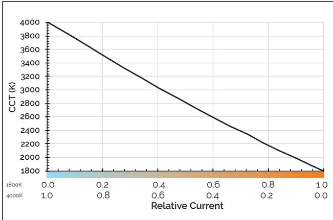
Figure 13: CCT Tuning Range,  $T_c = 85^\circ\text{C}$
