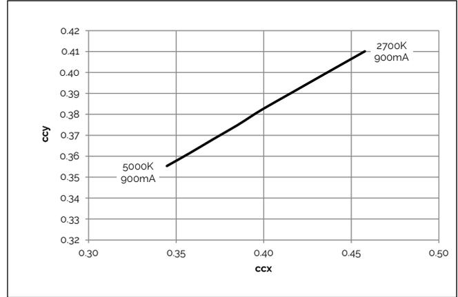
**Figure 14: CCT Tuning Range,  $T_c = 85^\circ\text{C}$**
