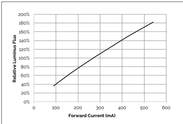
**Figure 14: V10C Typical Relative Flux vs. Current ( $T_c=25^\circ\text{C}$ )**
