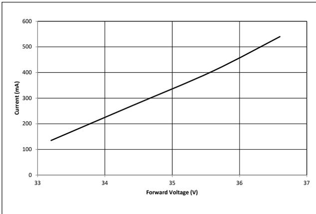
**Figure 12: V10C Drive Current vs. Voltage ( $T_c=25^\circ\text{C}$ )**
