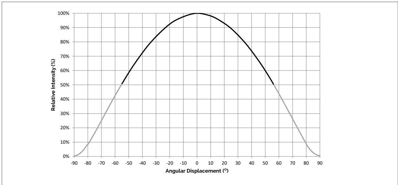
Figure 17: Typical Spatial Radiation Pattern
