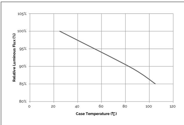
**Figure 4: Typical DC cxx Shift vs. Case Temperature**
