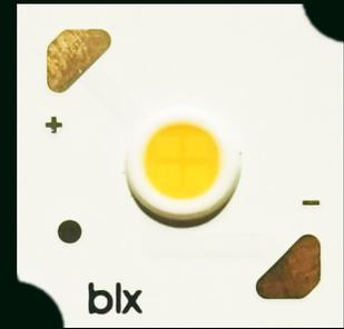
V Series™ HD LED array product, an ultra-high lumen density COB product line, is designed for high intensity spotlights used in commercial and retail settings. V Series HD arrays offer industry leading color over angle uniformity, and replace ceramic metal halide lamps by providing equal or greater center beam candle power at lower power and at greater lifetimes. Their tight beam control and exceptional quality of light is well suited for demanding directional spot applications.
