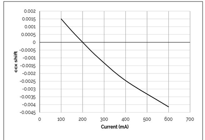
**Figure 9: Vero SE 10B Drive Current vs. ccy Shift**
