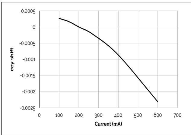
**Figure 10: Vero SE 10C Drive Current vs. ccx Shift**
