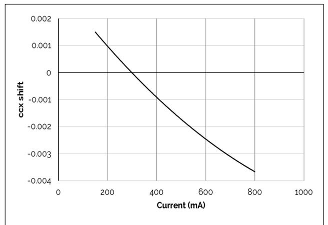
**Figure 11: Vero SE 10C Drive Current vs. ccy Shift**
