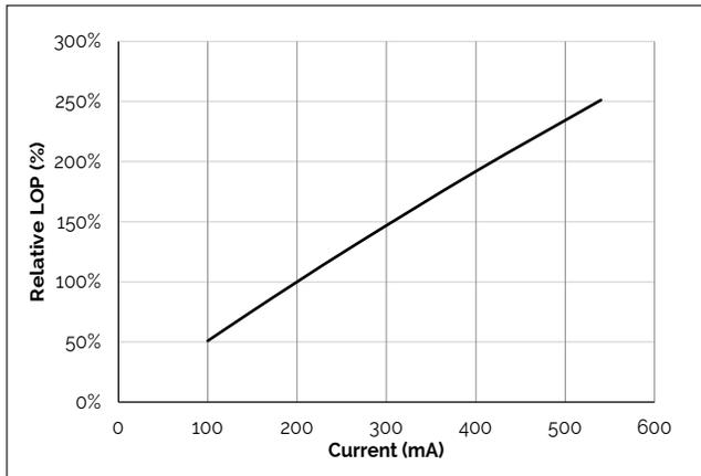
**Figure 4: Vero SE 10C Typical Relative Flux vs. Current**
