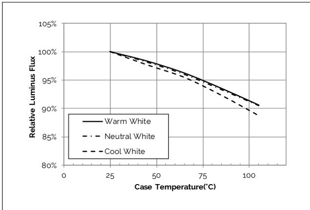
**Figure 18: Typical ccx Shift vs. Case Temperature**
