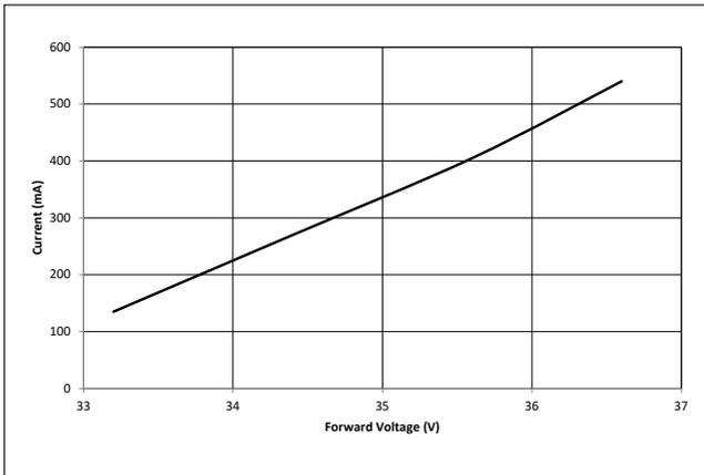
**Figure 12: Vero 10C Drive Current vs. Voltage ( $T_c=25^\circ\text{C}$ )**
