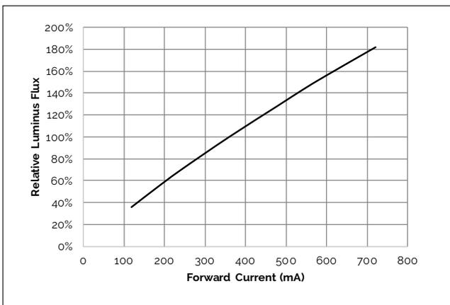
**Figure 16: Vero 10D Typical Relative Flux vs. Current ( $T_c=25^\circ\text{C}$ )**
