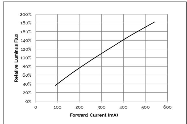
**Figure 15: Vero 10C Typical Relative Flux vs. Current ( $T_c=25^\circ\text{C}$ )**
