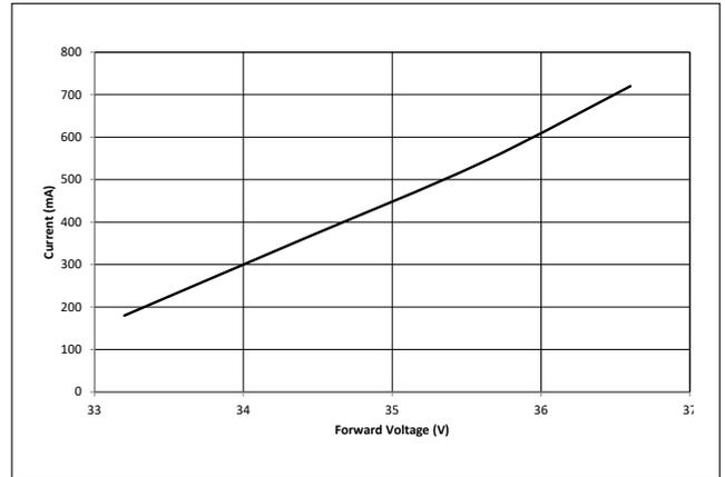
**Figure 13: Vero 10D Drive Current vs. Voltage ( $T_c=25^\circ\text{C}$ )**
