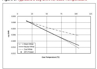
Figure 9: Typical DC ccx Shift vs. Case Temperature
