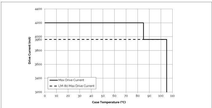
Figure 17: Vero SE 29D Drive Current Derating Curve
