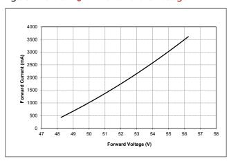
Figure 3: Vero SE 29D Drive Current vs. Voltage
