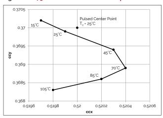
Figure 13: 5600K Color Shift vs. Case Temperature<sup>1,3</sup>
