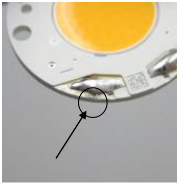
Figure 15a: Burnt or melted plastic due to the solder tip being held on the solder pad too long or due to the solder tip being too hot
