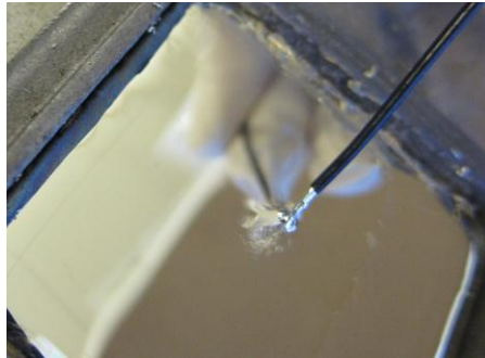
Figure 11b: Pre-tin the wire by dipping the tip of the wire in a solder pot
