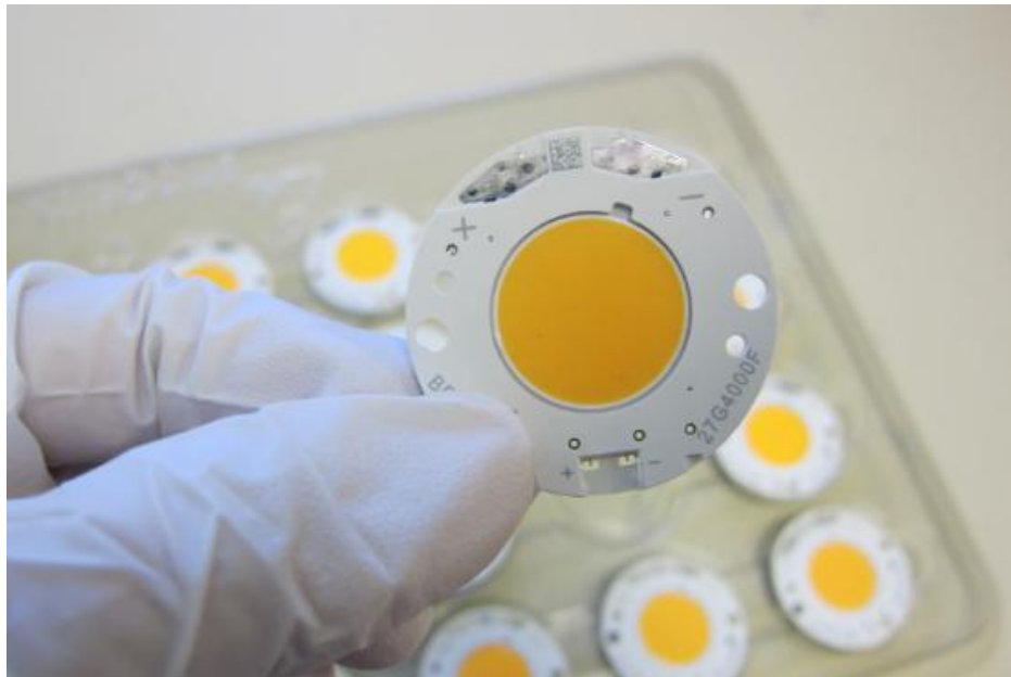
Figure 3: Wear gloves or finger cots when handling Vero LED modules from the plastic portion of the module
