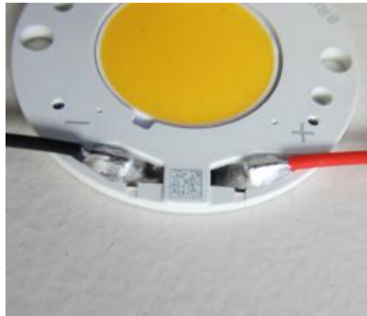
Figure 14: Good solder joints
