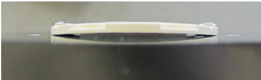
Figure 18: Typical Flex of Vero LED Module
