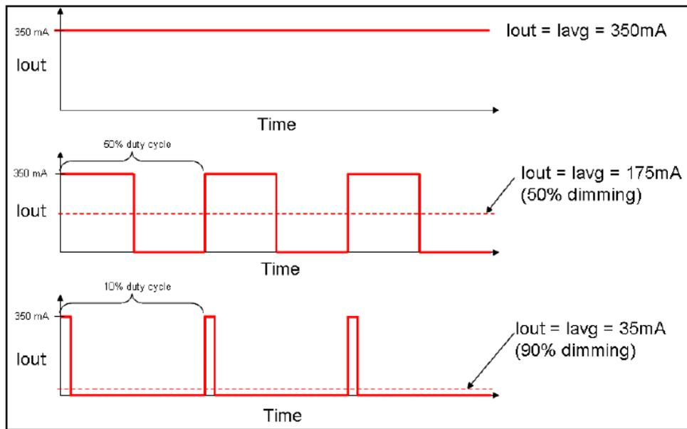
**Figure 7: PWM dimming to LED output**
