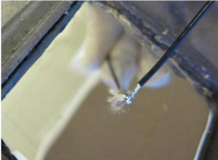
**Figure 17: Tinning pot – the preferred way to cleanly tin stranded wires**
