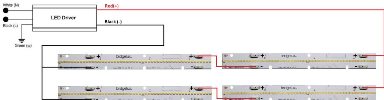
**Figure 6: Showing two sets of two EB Series modules in Series Configuration, in parallel.**
