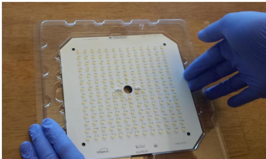
**Figure 14: Removal of EB Series Square module from tray**
