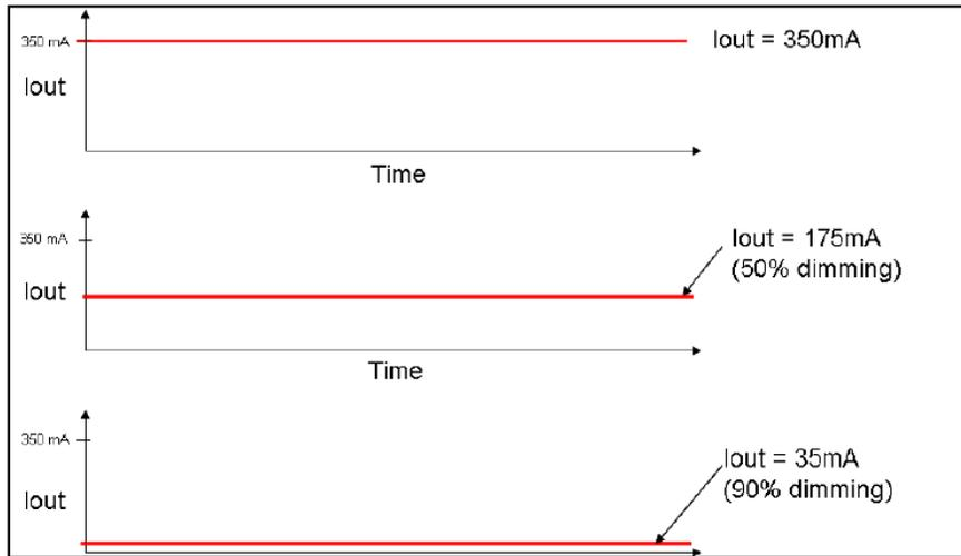
Note: A linearly dimmed current level does not bear a linear relationship to the actual light output (LOP) level of a LED and therefore the dimmed current percentage does not necessarily correspond to the same percentage of LOP reduction versus the maximum LOP level at 100% current level.
