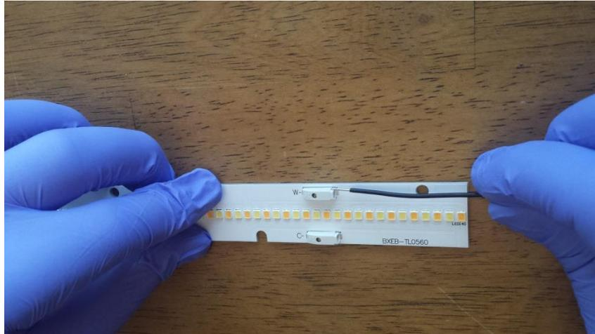
**Figure 18: Wire insertion by hand**
