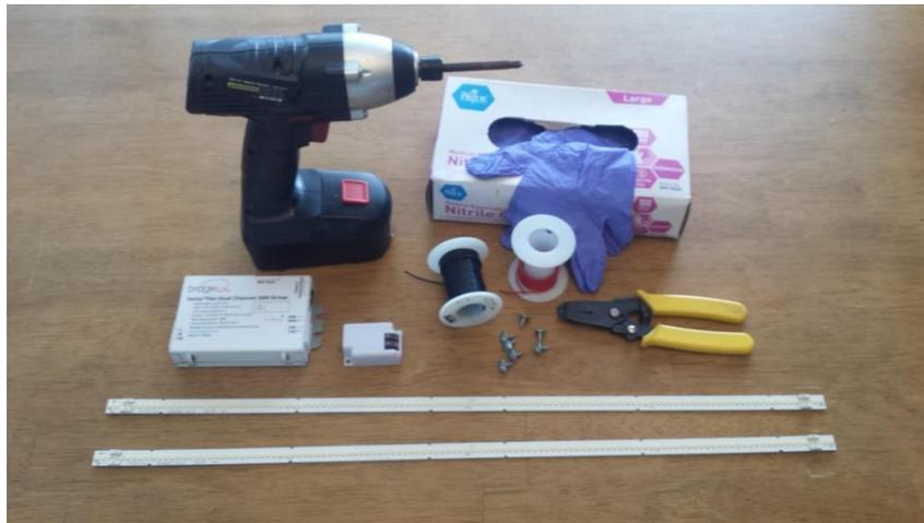
**Figure 11: Required tools – Bridgelux modules, wire, wire strippers, hardware, gloves, and drill. Not shown: glasses and goggles.**
