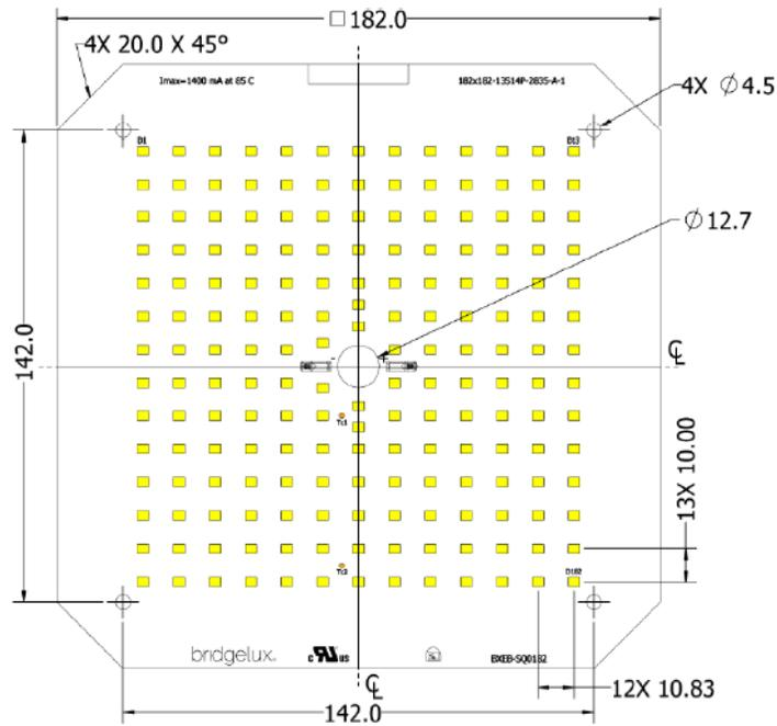
**Figure 2: Small EB Series Square module, ideal for the small parking garage light**
