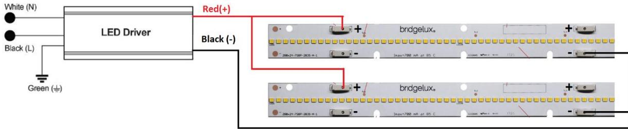
**Figure 4: Two EB Series modules in Parallel Configuration**
