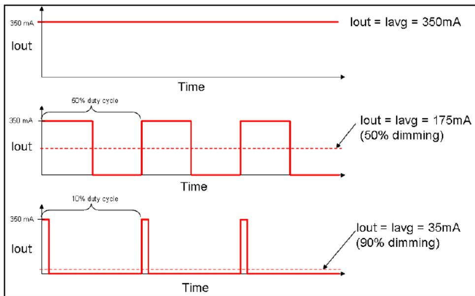
**Figure 7: PWM dimming to LED output**
