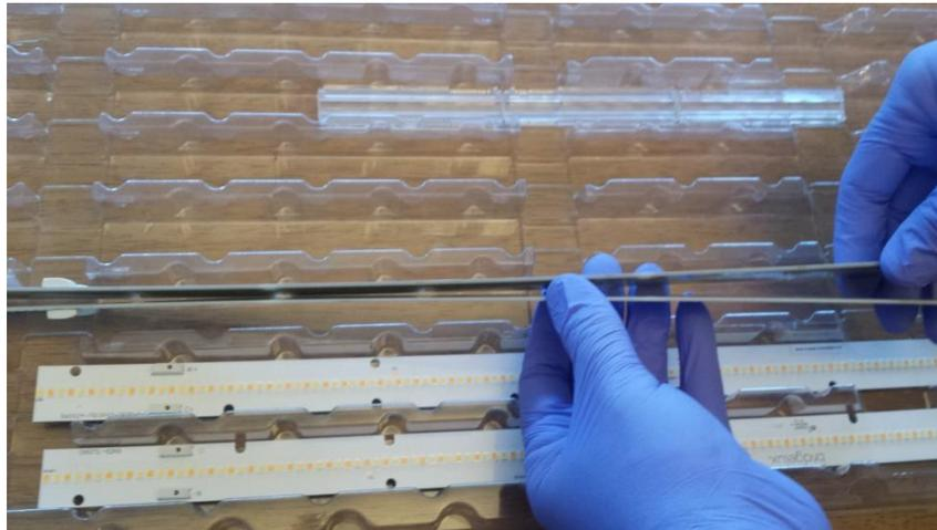
**Figure 15: Removal of a Vesta Linear Modules from tray**
