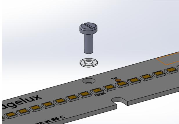
**Figure 21: Plastic, or insulating washers, can be used to help maintain clearance distances**
