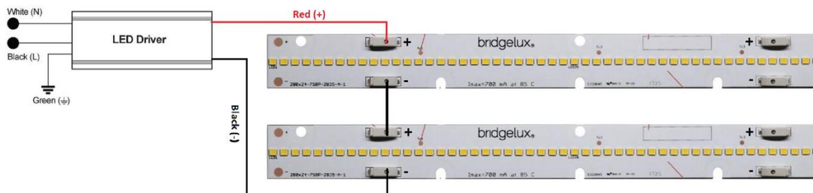
**Figure 3: Showing Two EB Series modules in Series Configuration**
