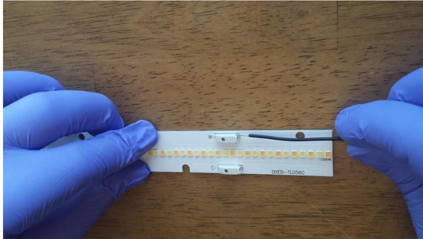
**Figure 18: Wire insertion by hand**
