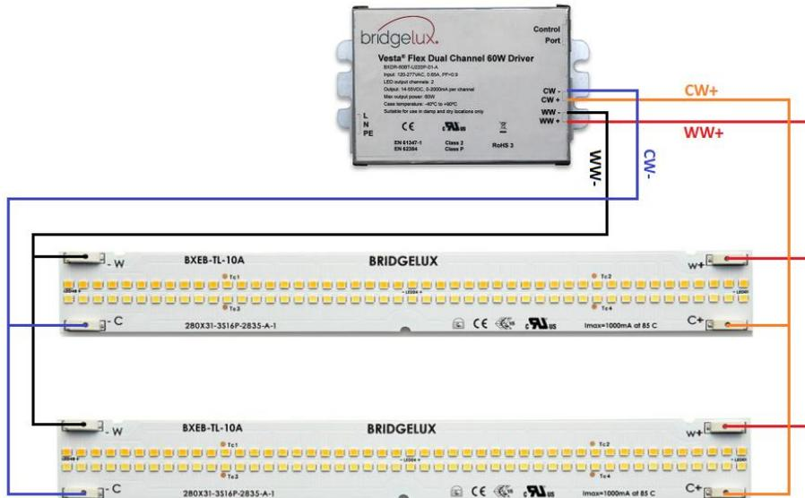
**Figure 5: Vesta Tunable White modules in parallel configuration on Bridgelux's Vesta® Flex driver.**
