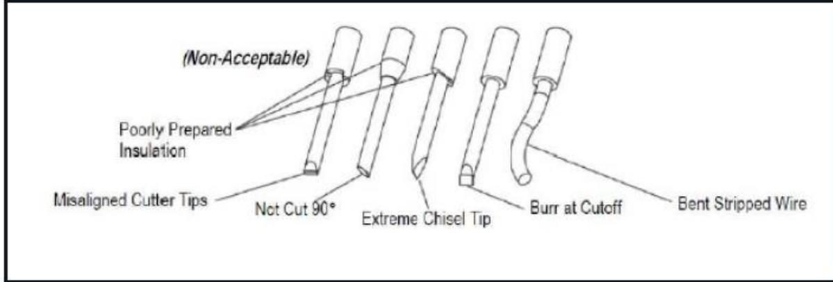
**Figure 16: Examples of unacceptable wire cuts**
