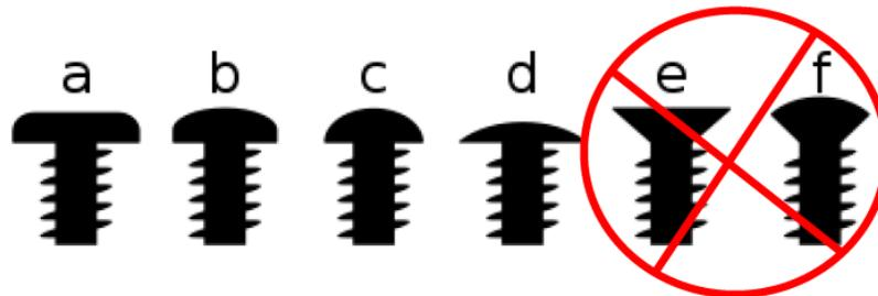
**Figure 20: pan head, button head, round head, and truss head screws are acceptable options**
