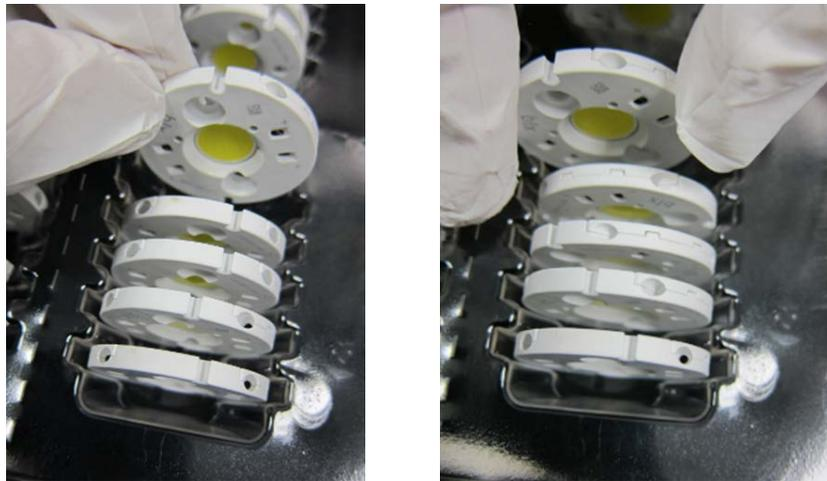
It is recommended to wear finger cots or gloves to prevent dirt or other contaminants from adhering to the Vero SE array (see Figure 2). Bridgelux Vero SE arrays are optical devices. Do not touch the optical area of the Vero SE array or apply stress to the yellow phosphor resin area. Contact may cause damage to the array. Do not bend the Vero SE array, as this can damage the product.
