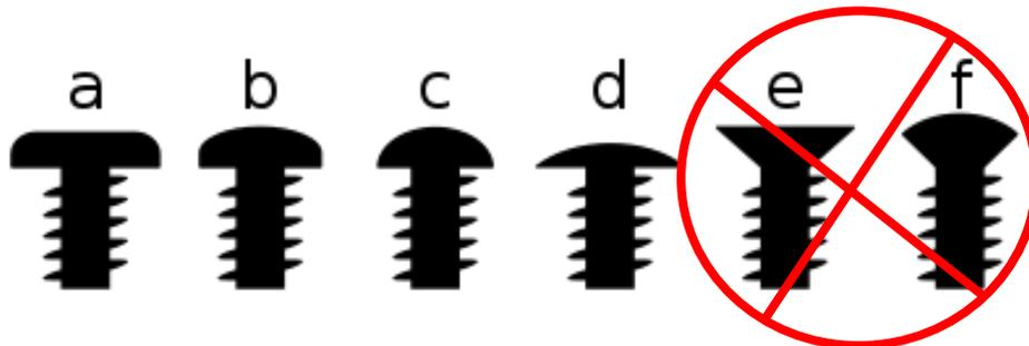
When selecting a screw, consider screws that have a low profile screw head that will fit within the Vero SE counter-bore so that the screw head will not block the light emitted from the Vero SE array. Additionally, if a secondary optic is to be used in the application, the screw head will be recessed within the counter-bore and not have mechanical interference with the optic.
