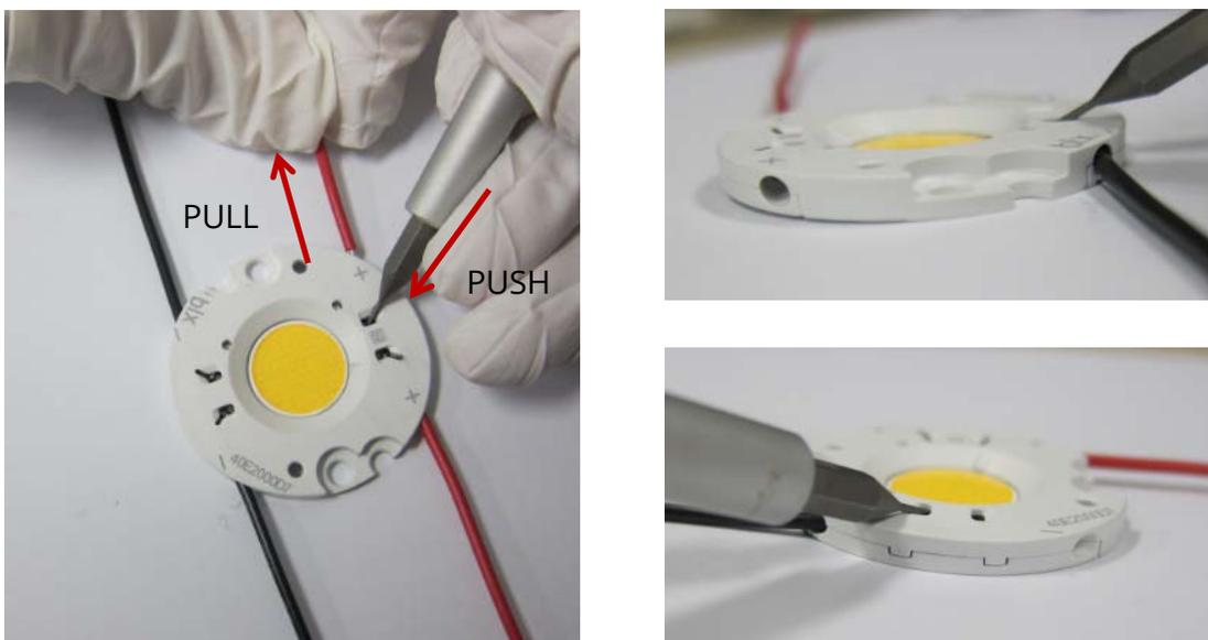
To release a wire from the wire trap, the wire must be pulled out at same time that the pressure is applied on the leaf spring. Note that the screwdriver tip is always angled toward the wire that is being released. Although not clearly visible in the pictures above, the screwdriver tip should come in contact with the leaf spring that is visible in the wire release mechanism port. **Wire may be removed up to three times from the wire trap.**
