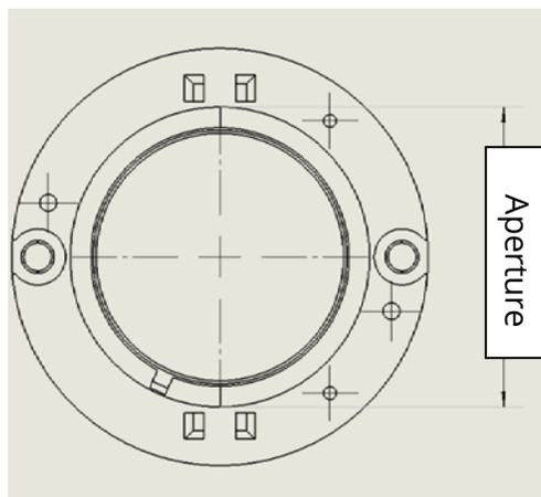
Although the LES dimensions are the same as standard Vero® Series and V Series™ array products, the apertures are larger. When requesting optics to test on the Vero SE, look for products that have apertures that are the same or larger than those aperture dimensions listed in Table 5.
