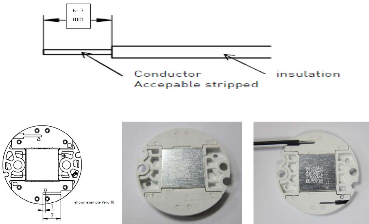
Note: The back of the Vero SE arrays have indentations, like those shown on the drawing above and in the middle picture, indicating the length wire should be stripped. The picture on the right hand side has had the indentations marked with black ink to make them easier to see.
