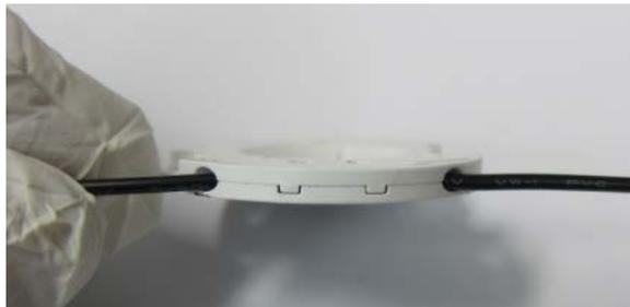
Please note that both the positive wire ports are electrically connected, as are the negative wire ports. See Figure 10 for details.
