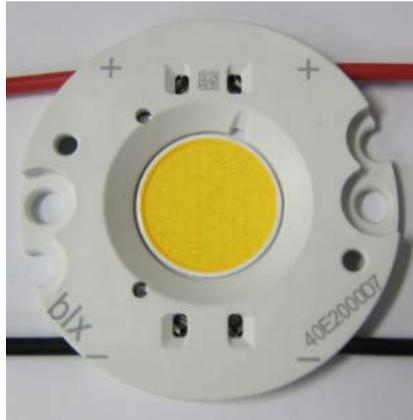
Because the wire ports are electrically connected, there are three possible wire configurations for the Vero SE arrays. These are shown in Figure 11.
