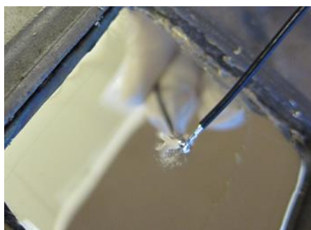
Figure 7b: Pre-tin the wire by dipping the tip of the wire into a solder pot
