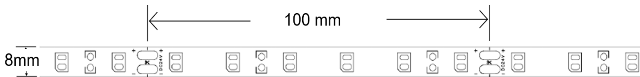
Figure 8: Drawing Overview for ECO LED Strip BXST-B1205-10xxE310C25-Axx
