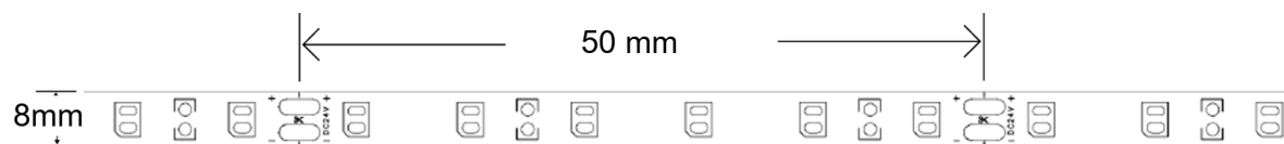
Figure 5: Drawing Overview for ECO LED Strip BXST-B1208-05xxE305C50-Axx
