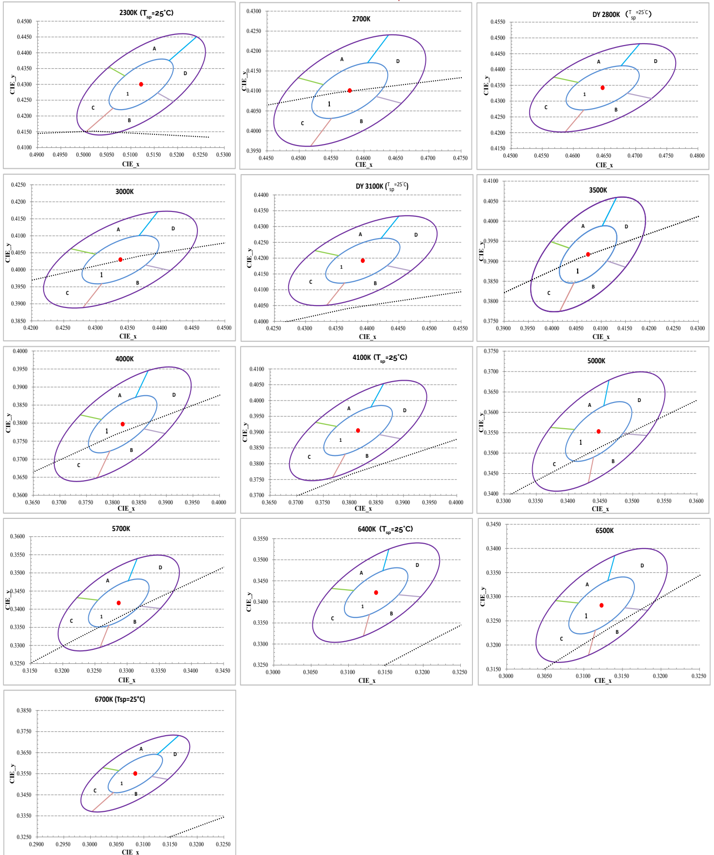
Figure 1: C.I.E. 1931 Chromaticity Diagram (5 Color Bin Structure, Hot-color Targeted at T_{sp}=85^{\circ}\text{C} , 2300K/DY 2800K/DY 3100K/4100K/6400K/6700K at T_{sp}=25^{\circ}\text{C} )
