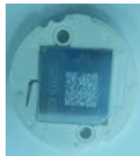
Step 2. Align COB under retaining lever, and rotate directly down into holder
