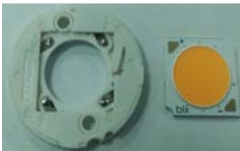
Step 1. Orient electrical contacts correctly - see wiring diagrams
