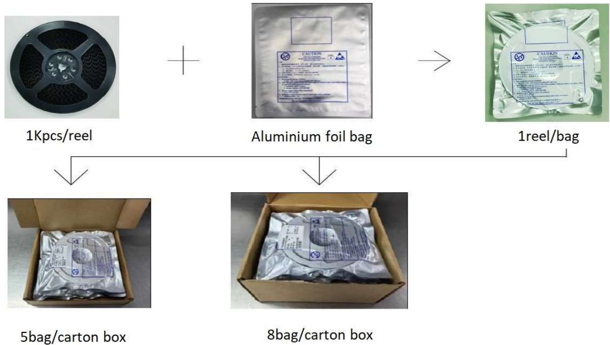
Figure 12: Emitter Reel Packaging Drawings
