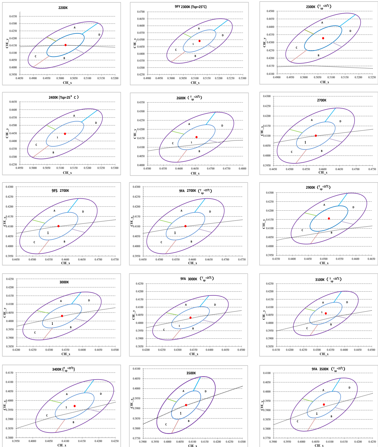
Figure 1: C.I.E. 1931 Chromaticity Diagram (5 Color Bin Structure, T_{sp}=85^{\circ}\text{C} , FY 2300K/2300K/2400K/2600K/ 9FA 2700K/2900K /9FA 3000K/3100K /3400K/ 9FA 3500K/3900K/9FA 4000K/4100K/9FA 5000K/ 5100K/9FS 5100K /6000K/9FA 6500K/6600K /6700K/9FS 6700K at T_{sp}=25^{\circ}\text{C} )
