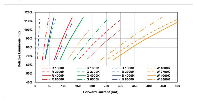
Figure 4: Typical Relative Luminous Flux (White CCT) vs. Drive Current Per Channel at CRI 95
