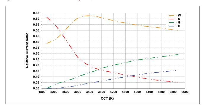
Figure 2: Relative Current Ratio vs. CCT at CRI 95 (T<sub>c</sub>= 85°C)
