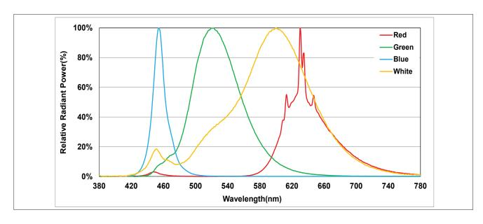
Notes for Figures 9 & 10: Color spectra measured at nominal current for  $Tc = 85^{\circ}C$ .
