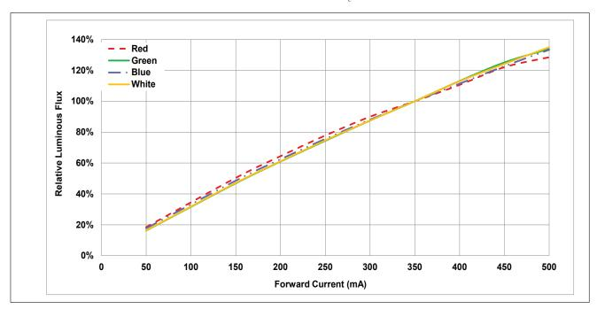
Figure 5: Typical Relative Luminous Flux (RGBW) vs. Drive Current Per Color (T<sub>c</sub>=25°C)
