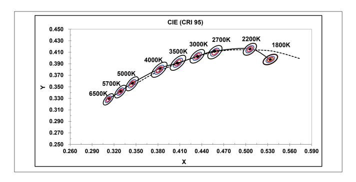
Figure 9: Typical Color Spectrum (White CCT, at  $T_c = 85^{\circ}$ C)
