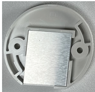
Step 2. Align the Array and push straight down to holder cavity, face the side with connectors toward the opening of the holder.
