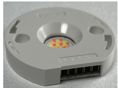
Completed Array and holder
