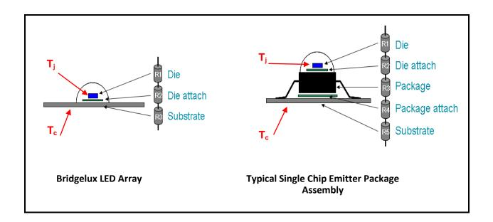
Fig 1: Comparison of thermal path for Bridgelux LED Array and a typical single chip emitter package
