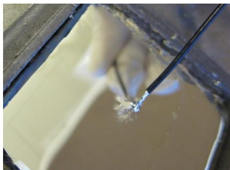
Figure 4b: Pre-tin the wire by dipping the tip of the wire in a solder pot
