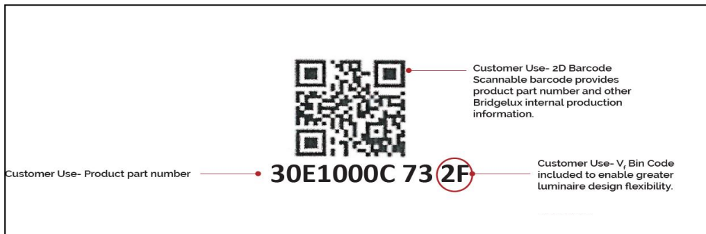
Figure 13: Markings on the back of the Gen 7 array which identify the V_f bin of the array.
